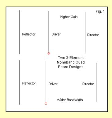
The wide-band version is about 19% longer than the high gain model. Despite the greater length, the wide-band driver is closer to the reflector than the corresponding element on the high-gain version. The wide-band director is also considerably smaller in circumference than the high-gain director.
