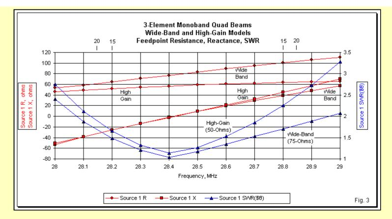
The wide-band resistance curve centers at about 75 Ohms. Although the resistance change across the band is higher than the corresponding change for the high-gain model, the reactance shows a much lower total change from 28 to 29 MHz. Hence, the wide-band models shows a 75-Ohm SWR curve that covers about 900 kHz of the band with less than a 2:1 value. The same curve on 20 and 15 meters would show band-edge values well below 2:1.
